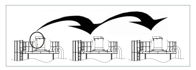
In case of plants with many filters, WAM® suggests using a single tube to be shifted from one filter to another. After making the measurement, remove the tube and air closure plates.
