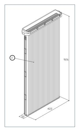
The SILOTOP® zero dust collectors feature POLYPLEAT® filter elements.
